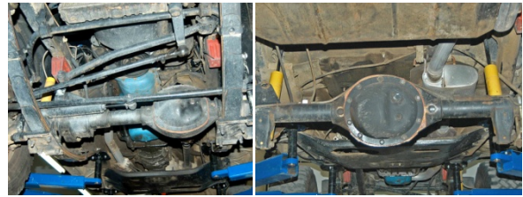
Four- and six-cylinder YJ frames have different part numbers. Shown is an '87 Wrangler chassis with a 2.5L four, the AX-5 transmission, a Dana 35 rear axle and an NP207 transfer case.
