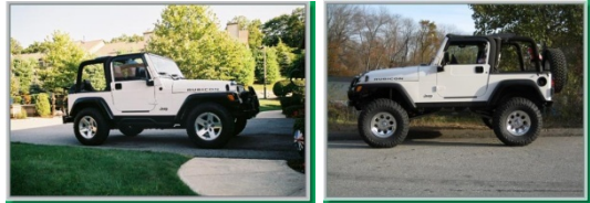
Before and after poses of the '04 TJ Rubicon—6-inch lift is clearance for 35" diameter Toyo tires. (Photos by Joe M.)
