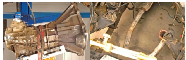
2.5L's AX-5 transmission is weaker than AX-15 used with sixes. Output spline count differs, too. Note motor mount positions on the frame rails. Six-cylinder mounts are further forward.
