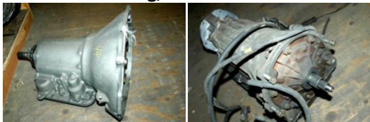
Stock 3-speed Jeep automatic (left); AW-4 core (right).
