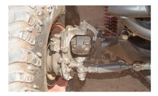
A growing interest in reduction and dropped front axles, mostly from military surplus sources, has created the ultimate rockcrawling setup. Primary advantage is ground clearance at the differential housing.
