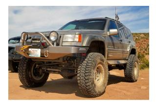
This ZJ Grand Cherokee has been modified extensively for serious off-pavement use. A trail runner and on-highway cruiser, this is the quintessential multi-purpose machine, boasting a V-8 engine and the kind of axles, transfer case and gearing typically found on radically modified, trail-prepped Wranglers.
