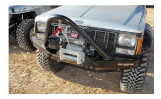
Full-Traction Suspension's XJ Cherokee twodoor targets an increasingly popular off-road market. Retrofit axles with lockers, big tires, a six-inch FTS long-arm suspension lift, Hanson steel products and a Warn winch have created a formidable trail runner. Used XJs can provide an affordable starting point.
